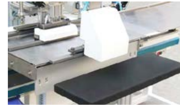
自动整齐收料装置 Automatic neat receiving device
