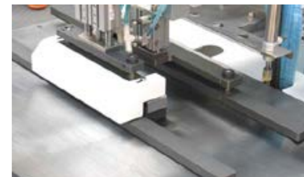
布料卷边定位、确保脚边平齐 Position fabric hem and make sure foot edge is flush
