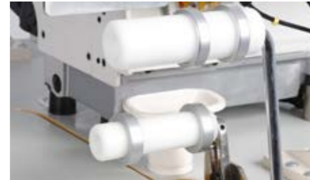
气动滚轮扩张器，轻松上料 Pneumatic roller expander for easy feeding
