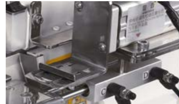
拉筒式气动卡位装置让缝迹左右对齐圆领宽度一致 The tubble-type pneumatic clamp allows the seam to be aligned to the left and right of the collar to be the same width
