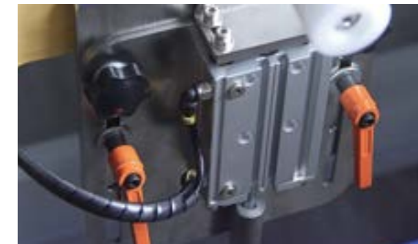
扩张器设计方便调节罗纹松紧度 The expander is designed for easy adjustment of rib tightness
