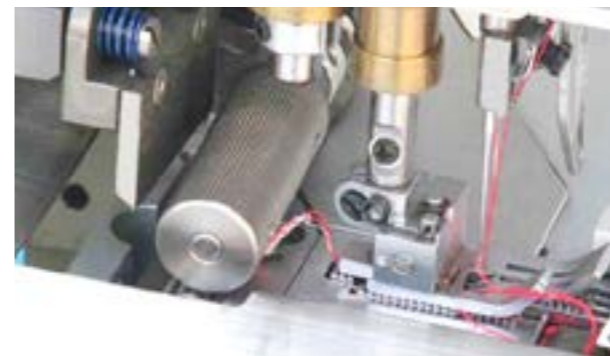
车缝完自动剪线 Automatic cutting after sewing
