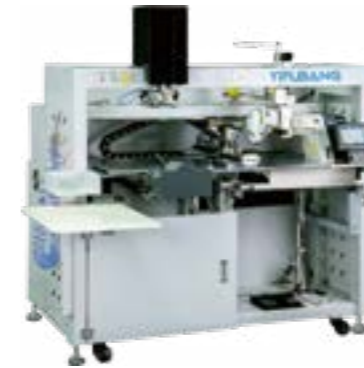
JCL1L 全自动衬衫左袖叉工作站 Automatic left shirt sleeve placket attaching machine
