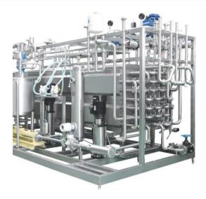
Soya milk production line is mainly used to produce soya milk products, etc. This line uses raw soya bean or soya powder as raw material. After pasteurizing and homogenizing, the final products are of flavored taste. Most important of soy milk plant is to remove the bean smell, and the vacuum deaerator is surely necessary. Additionally, we can design production lines in accordance to the customers' requirements.
