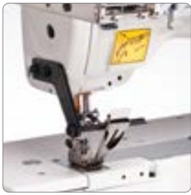
FWP 附喇叭 (B417R) 与导带架 With folder (B417R) and tape guide.
