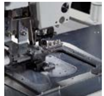
FZ 反转压脚 Inverted Clamp
