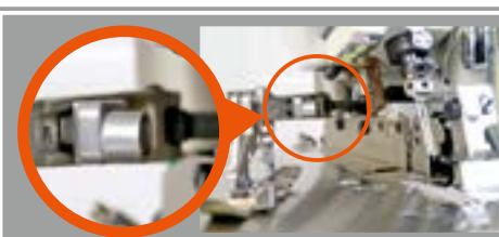
抬压脚安全感测装置 Presser Foot Lift Sensor
