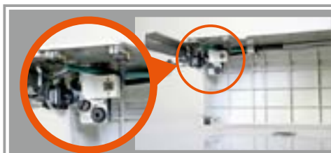
布盖板安全感测装置 Cloth cover safety sensor
